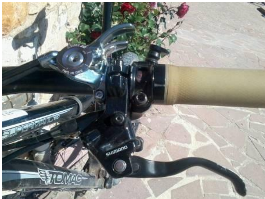
2 in 1 trigger remote dtswiss lockout for both lock- release front-rear suspension
